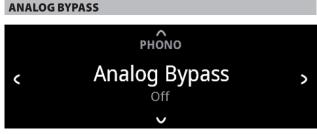
All analog signals remain in the analog domain without analog-to-digital conversions.
