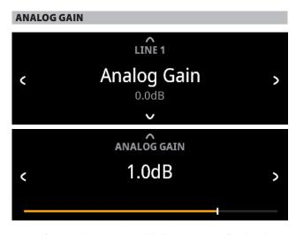
Use front panel [</>) or SR 10's [¶/₱] buttons to set preferred Analog Gain level.
