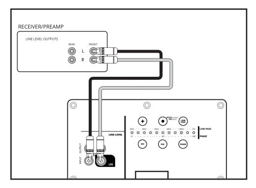
Enable and adjust the on-board low pass filter of the PB-3000 for a smooth blend with the main speakers.
