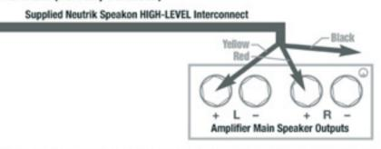
NOTE: The Serie S models are equipped with internal circuitry to allow seamless connection to Class-D (digital) amplifiers. If connecting to a Class-D amplifier, follow the above connection procedure for differential amplifiers.
