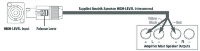
For differential (i.e. fully balanced) amplifiers using one REL, simply use the standard connecting scheme
