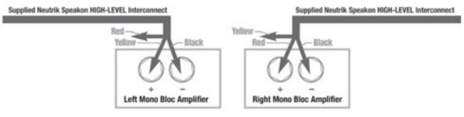
yellow wire from the twisted pair. This will reduce output by half and restore a natural dynamic. If the amplifier is of balanced differential design, please follow the instructions in the section above labeled Differential Connection.
