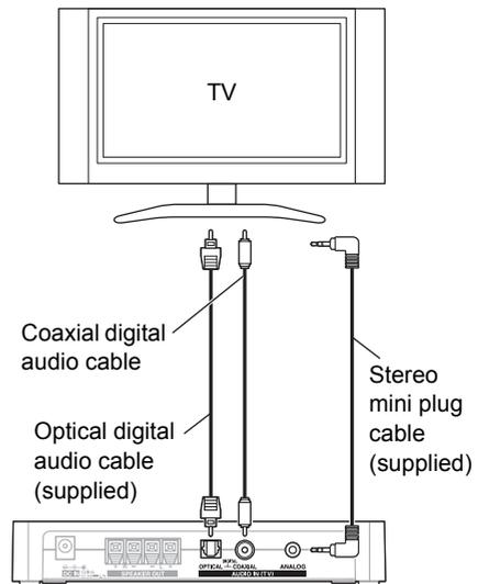
Connect the TV to either of the jacks of the controller.
