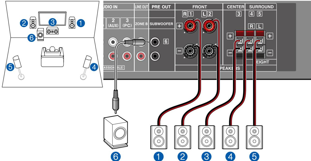
This is a basic 5.1 Channel System. For details of the speaker layout, refer to "Speaker Installation" (→p16).
