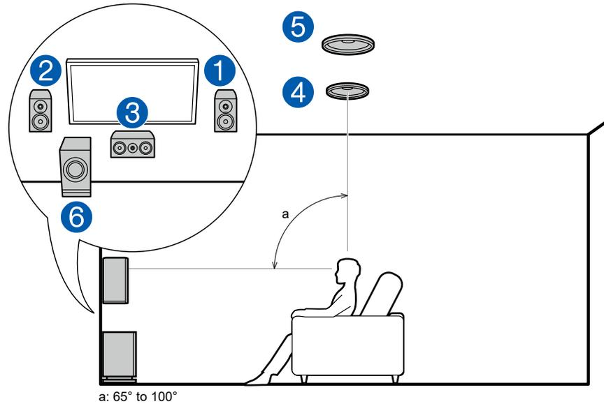
This is a 3.1-channel system consisting of front speakers, a center speaker, and a powered subwoofer, with the addition of top middle speakers, a type of height speaker. Installing the height speakers will enrich the sound field feeling in the upper space. Fit top middle speakers on the ceiling directly above the listening position. The distance between each pair should match the distance between the two front speakers.
