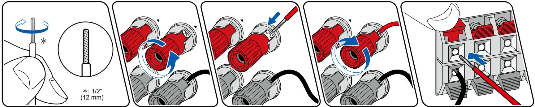
Make correct connection between the unit's jacks and speaker's jacks (+ side to + side, and - side to - side) for each channel. If the connection is wrong, a bass sound will not be reproduced properly due to reverse phase. Twist the wires exposed from the tip of the speaker cable so that the wires do not stick out of the speaker terminal when connecting. If the exposed wires touch the rear panel, or the + side and - side wires touch each other, a malfunction may occur.
