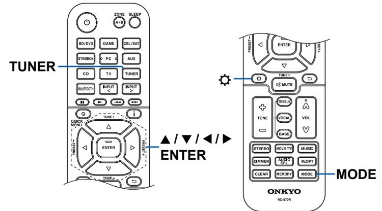
**When FM broadcasts reception is poor:** Perform the procedure for "Tuning Manually" ( →p38). Note that if you tune manually, the reception for FM broadcasts will be monaural rather than stereo, irrespective of the sensitivity of the reception.
