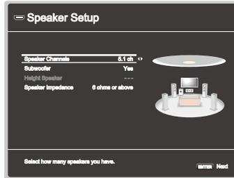
2. The speaker combination selected in step 1 is displayed. "Yes" is displayed for the selected speakers. If the setting is correct, press ENTER.
