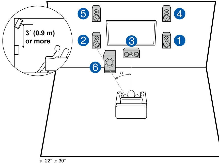
This is a 3.1-channel system consisting of front speakers, a center speaker, and a powered subwoofer, with the addition of front high speakers, a type of height speaker. Installing the height speakers will enrich the sound field feeling in the upper space. Front high speakers should be situated at least 3'/0.9 m higher than the front speakers.
