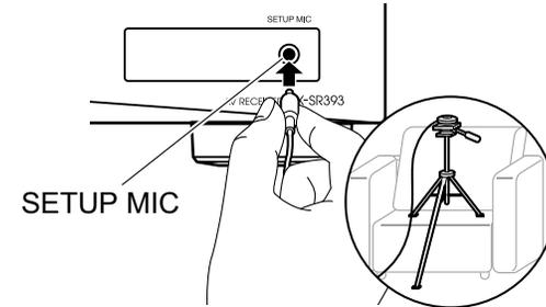
When placing the speaker setup microphone on a tripod, refer to the illustration.
