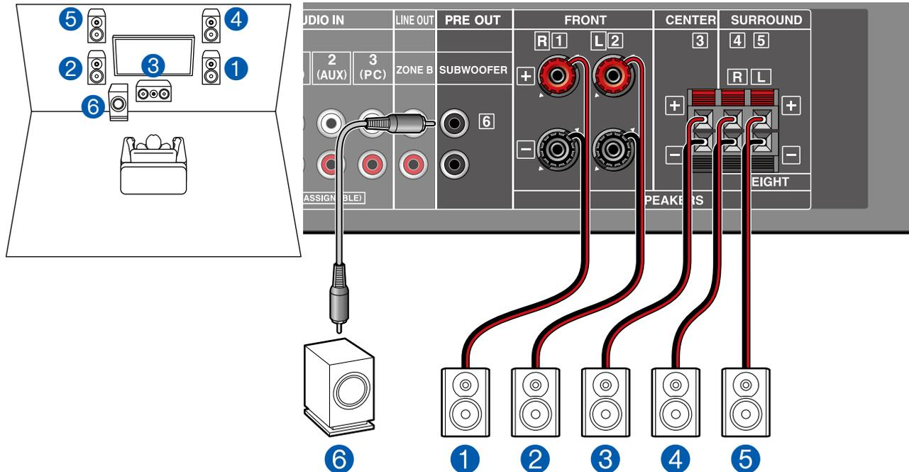
This is a combination of the 3.1 Channel System and front high speakers. A front high speaker is a type of height speaker. You can select only one set of height speakers from the following three types for connection.
