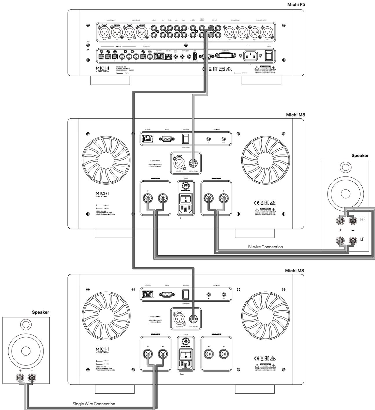
**Figure 4-1 : Balanced (XLR) Inputs Connection**
