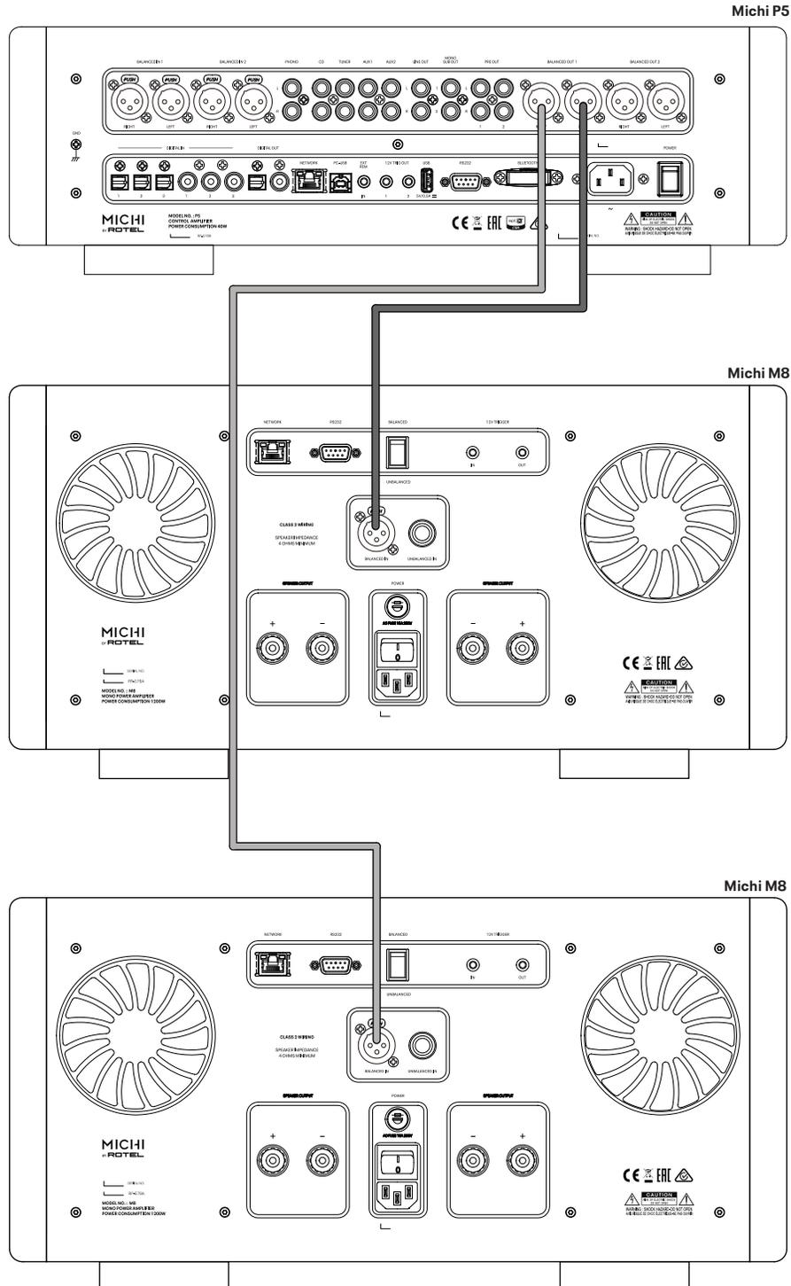
**Figure 5-1 : 12V Trigger Connections**
