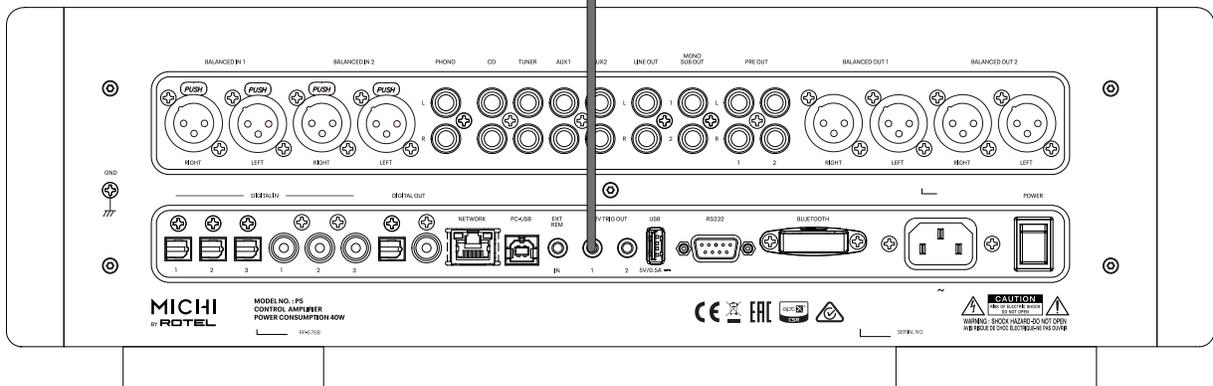
**Figure 5-2 : 12V Trigger Connections**
