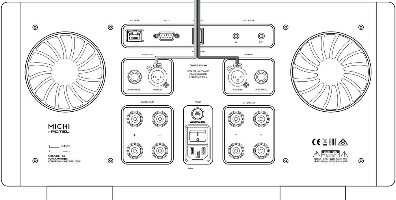
**Figure 4-2: Balanced (XLR) Inputs Connection**
