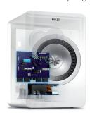
professional studio monitors, each speaker has two dedicated class AB amplifiers, one for LF/MF and one for HF. With each driver powered by its own amplifier, the tweeters (vented to reduce distortion) are unaffected when the woofers are driven close to the limit, resulting in greater control at a higher volume and a much cleaner sound.
