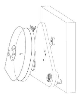
After the placing the record on the platter, it is necessary to tighten the screw-able record clamp (6) onto the platter spindle.
