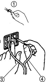
② Depress the terminal lever, and insert the tip of the cord into the hole and then release the lever so that it springs back into position.
