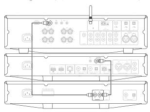
Adding an additional connection from CXN to CXA will enable the use of the StreamMagic app function.
