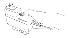
To disassemble, push latch outward to remove or replace plug.
