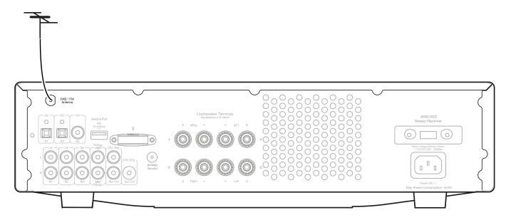
Note: The AXR100D is supplied with a temporary aerial for initial use. For permanent use, outdoor aerials are highly recommended.
