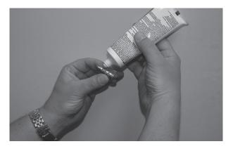
13 The left screw hole will require a drywall anchor. *Use glue* on the threads when installing this anchor to the drywall.
