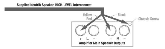
**NOTE:** The Habitat1 is equipped with internal circuitry to allow seamless connection to Class-D (digital) main amplifiers. If connecting to a Class-D amplifier, follow the above connection procedure for differential amplifiers.
