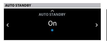
Auto Standby feature is an integral feature of C 399 that conforms to European ecodesign regulations. The C 399 can be setup to automatically go to standby mode if there is no user interface interaction and no active source input within 20 minutes.
