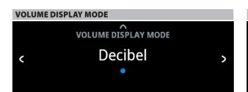
Volume Display Mode gives the user two options on how to display Volume level. Use  ${\sf C}$  or  ${\sf >}$  to select between "Decibel" and "Percent" Volume display mode.
