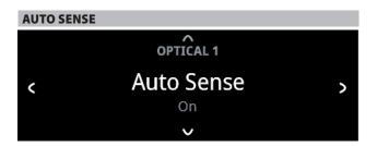
Auto Sense can be setup for each Source. Auto Sense feature enables the designated Source to wake up from standby mode when an active source is detected from the particular Source's input.
