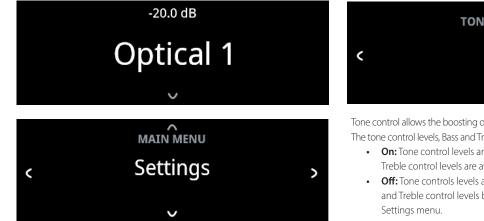
Press front panel [v] button once for the Main Menu options to appear in the display. Use front panel < or > button to select through the Main Menu options – **Settings, Source Setup** and **System Info**.
