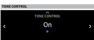
Tone control allows the boosting or reduction of particular audio frequencies. The tone control levels, Bass and Treble, can be turned on or off.
