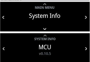
"System Info" displays information about current MCU, LCD and FPGA firmware versions.
