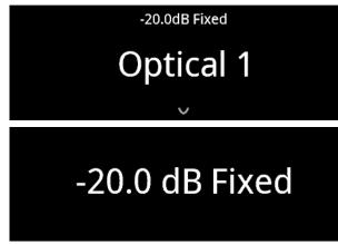
At Fixed volume level setting, front panel display will show "xx.x dB Fixed" as the volume control is adjusted.
